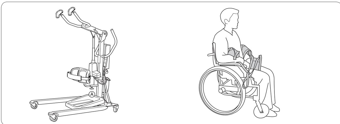
1. Disassemble the lower leg support: Unscrew screw A. Pull out the lower leg support. Remove the foot rest: Grab the front edge of the frame. Fold it up and lift it off the base.
