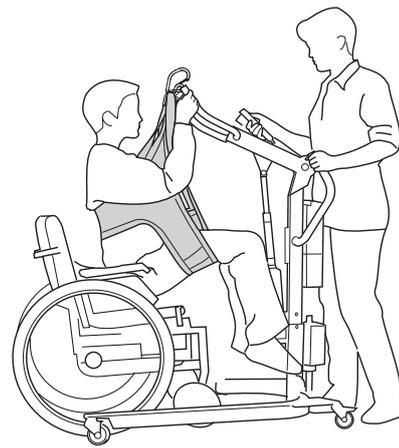
3. Advance the lift. Connect the sling's suspension loops to the sling bar's hooks. The height setting of the lift mast may have to be adjusted, see page 5.
