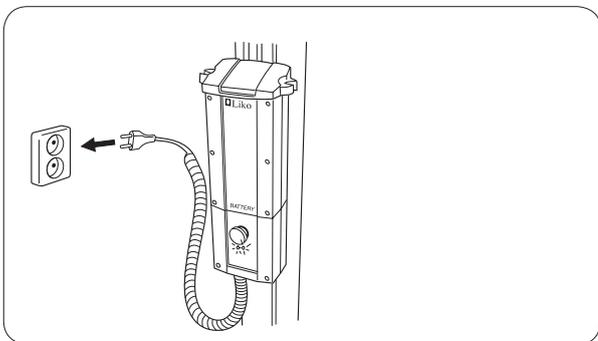
13. Before the first use, the lift's battery should be charged for at least 6 hours. For detailed instructions, see "Charging the Batteries", p. 8.
