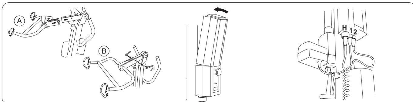
3. A) Remove the locking handle from the lift arm. Slide the sling bar onto the lift arm with the opening on the lifting hooks facing upward (see illustration). B) Attach the locking handle and tighten.
