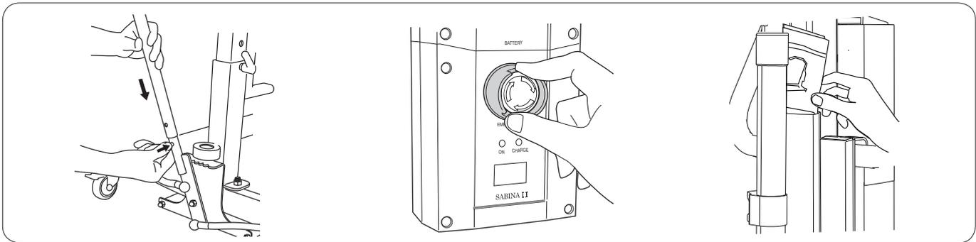
10. Install the lever for base-width adjustment (only Sabina II EM): Push in the catch on the lift and put the lever in place. Rotate the lever to the right position (a clicking sound will be heard).
