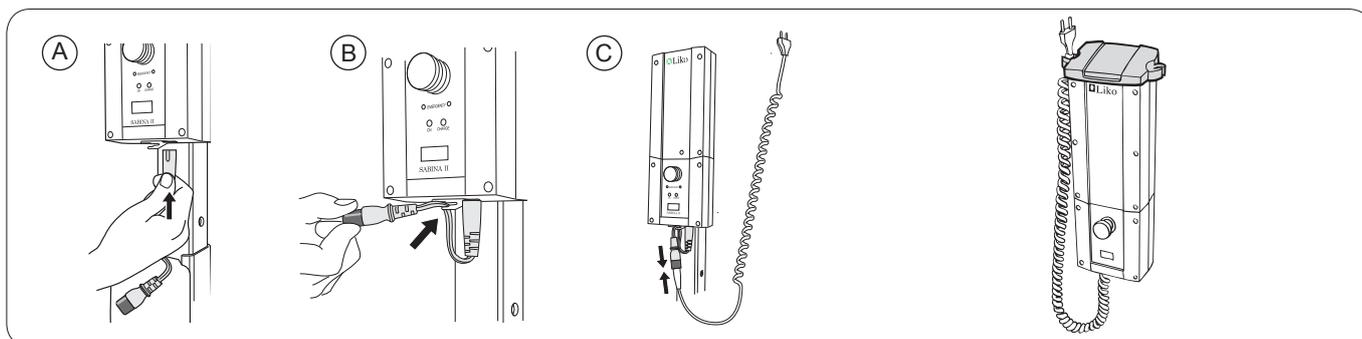
6. A) Connect the charger cable to the socket under the control box.
