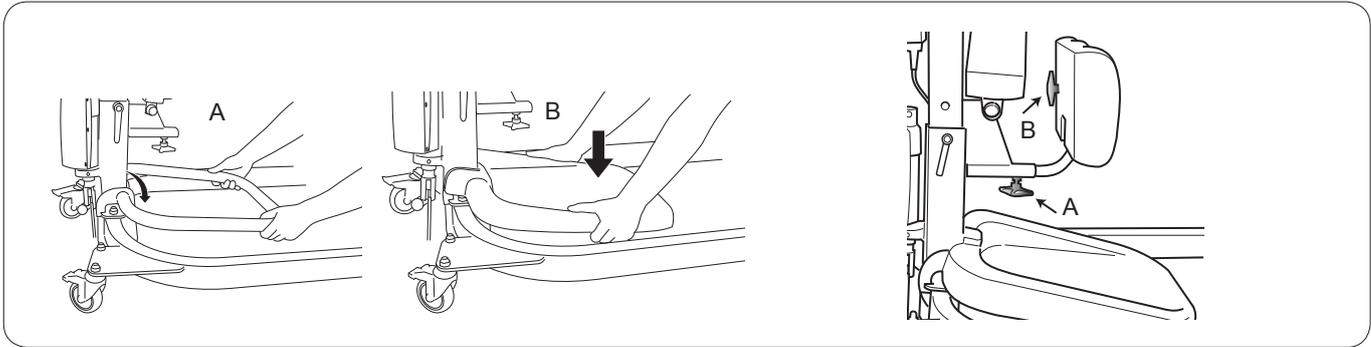
8. A) Put the frame for the foot rest over the lift mast's bracket to the base. Make sure the frame is securely in place.
